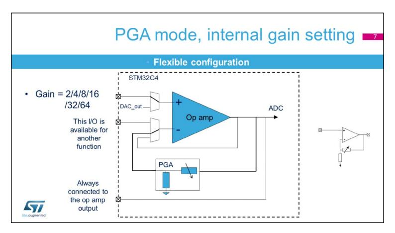
The op amps support non-inverting amplifier mode with **six** fixed gains available. The feedback resistors can be selected to have gain of 2, 4, 8, 16, 32 or 64 to support the Programmable Gain Amplifier function. It may also be beneficial to use the op amp as an ADC input so that the full dynamic range of the analog-to-digital converter can be applied to signals having a small amplitude.
