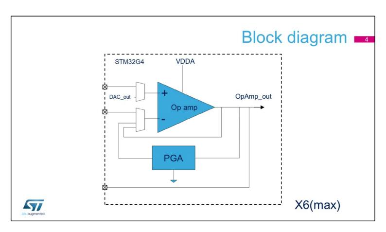
This slide shows the block diagram of the operational amplifiers. The STM32G4 integrates up to six operational amplifiers. Several switches are used to configure different functions. Each op amp can be configured individually.
