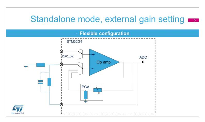
The operational amplifiers support this default configuration using the factory trimming values and operate in normal.
