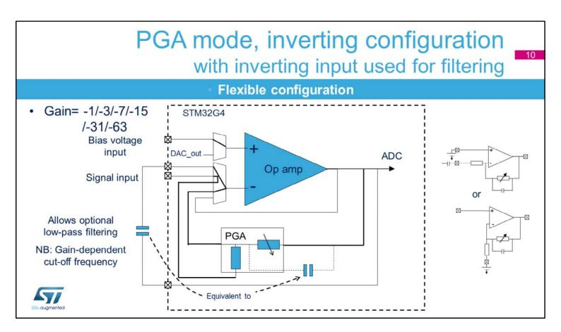
The op amps also support external connections on outputs and on the inverting input also for this PGA mode. It enables the connection of an external capacitor to add low-pass filter characteristics to the PGA configuration.
