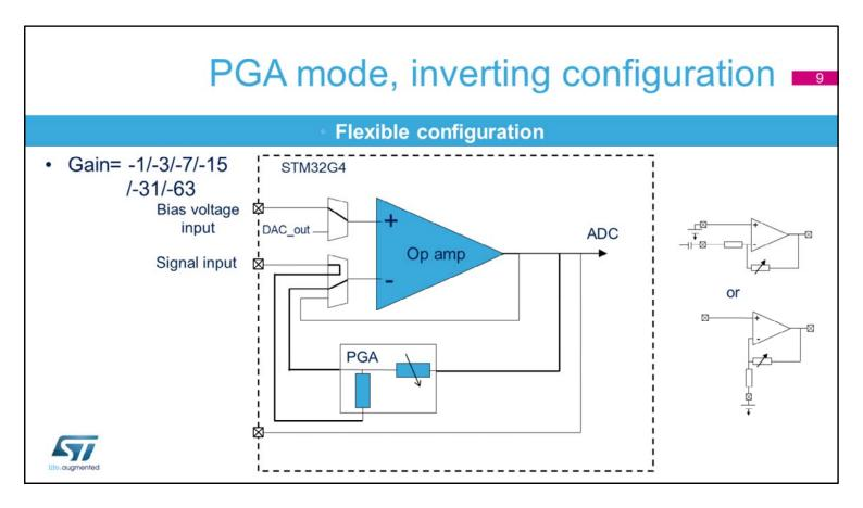
This STM32G4's op amps support inverting amplifier mode with six fixed gains available. The feedback resistors can be selected to have gain of -1, -3, -7, -15, -31 or -63 to support the Programmable Gain Amplifier function. By using this configuration, it is possible to shift the bias voltage of the input signal with AC coupling capacitor. It can also be used as a non-inverting amplifier with a gain of 2, 4, 8, 16, 32 or 64 with bias to a none ground voltage.
