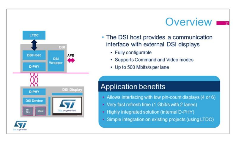
The DSI Host integrated inside STM32 microcontrollers provides a high-speed communication interface allowing the microcontroller to communicate with a display with a reduced pin count. This interface is fully configurable, making it easy to connect DSI displays available today on the market.
