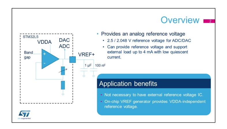
The VREF buffer embedded into STM32L5 microcontrollers provides a stable voltage based on an internal bandgap reference for use by both the analog-to-digital and digital-to-analog converters. Its output voltage is programmable to 2.5 or 2.048 V. This output voltage can also support external loads up to 4 mA. External bulk and bypass capacitors are required when the internal VREF buffer is used.
