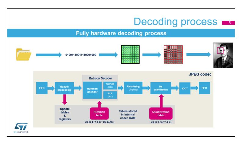
The decoding process follows the JPEG baseline algorithm: The file data are sent to the input FIFO. The file header is parsed and the corresponding internal RAM tables are updated. Once the header has been parsed, an interrupt can be raised. The compressed data are sent through the entropy decoder to generate the 8 by 8 Minimum Coded Units (MCUs) using the zigzag ordering. The resulting 8x8 tables are de-quantified and transformed through an inverse DCT (iDCT) into the original picture data.
