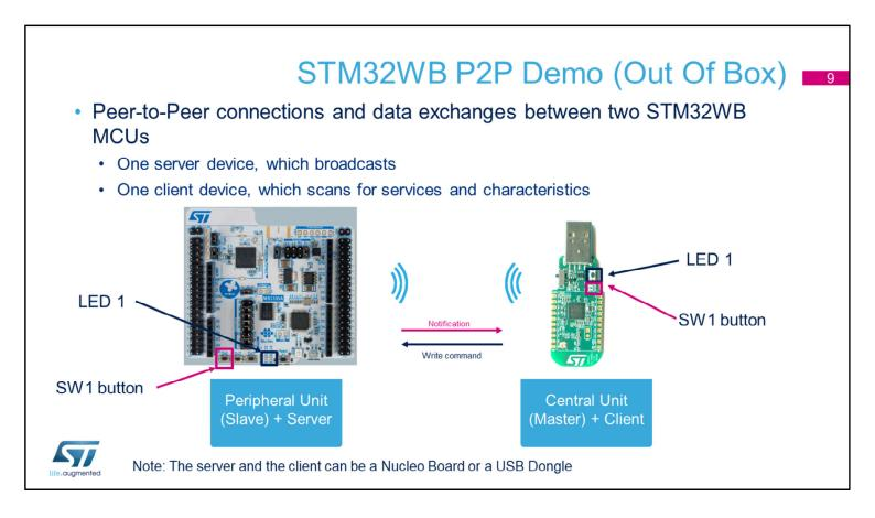
This peer-to-peer demo uses both the Nucleo board and the dongle.
