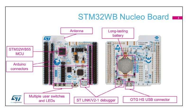
This is the STM32WB55 Nucleo board. It offers several connectors for power and 2 USB peripherals. Multiple user switches and LEDs are also available.
