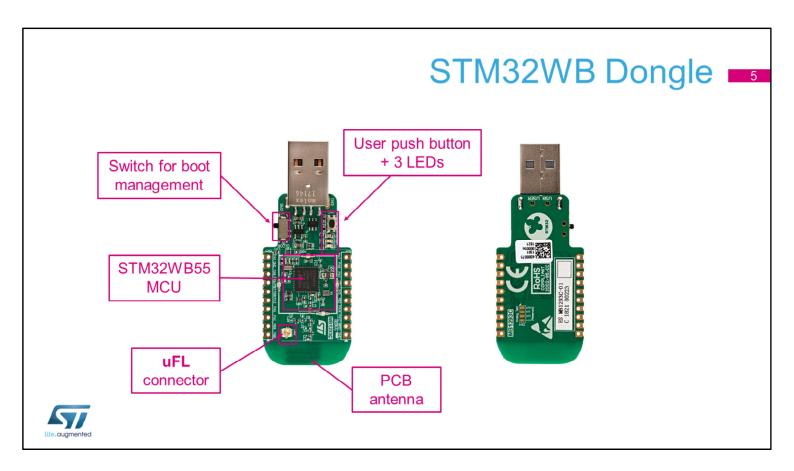
This is the STM32WB USB dongle. It is a 2-layer PCB with a user push button and three user LEDs.
