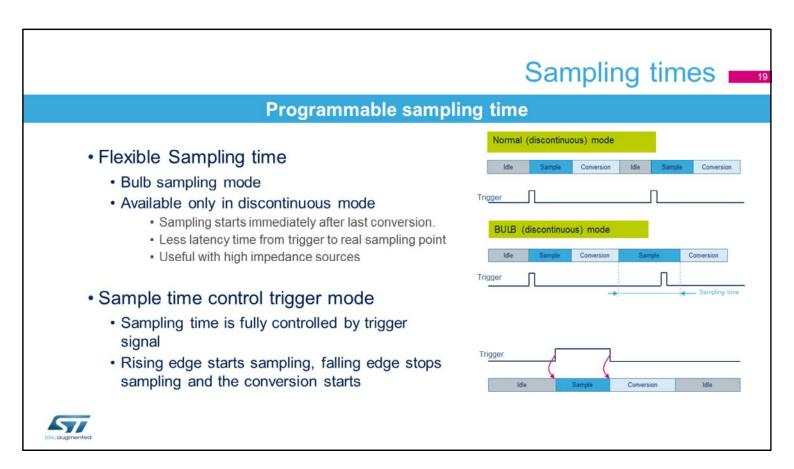
Two new sampling mechanisms have been introduced. The first one is the bulb mode which works only in discontinuous mode.
