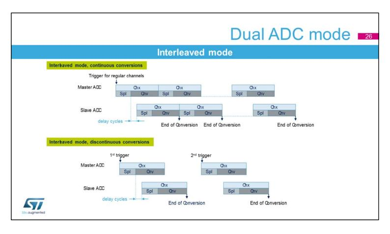
Interleaved mode converts a regular channel group (usually one channel).
