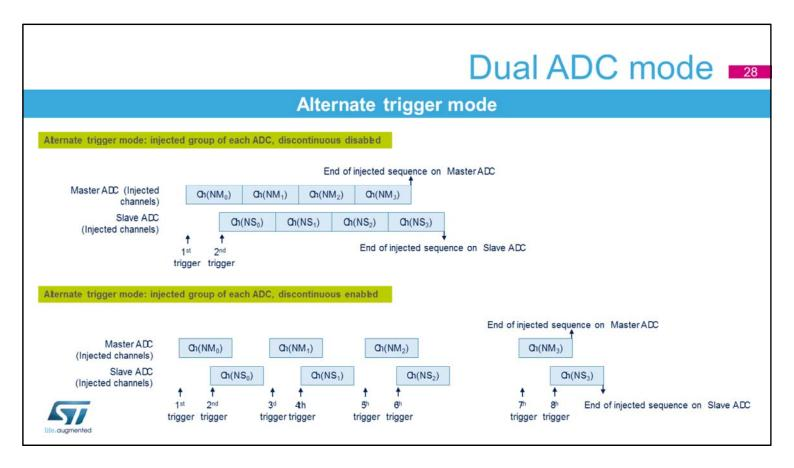
The Alternate Trigger mode converts an injected group of channels.
