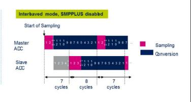
When a sampling time of 2.5 ADC clock cycles is selected, the total conversion time becomes 15 cycles in 12-bit mode.
