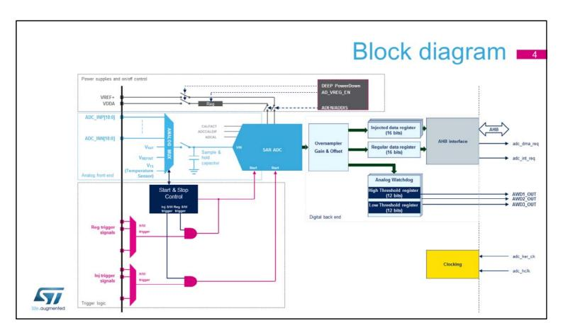
This slide shows the general block diagram of the ADC. The main important sub-units of the ADC are:
