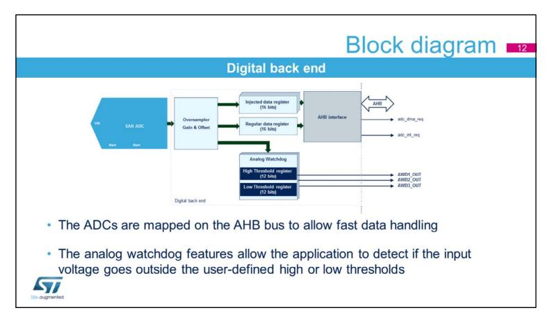
The digital back-end performs processing on the samples obtained in the SAR ADC in the over-sampler, gain & offset unit.
