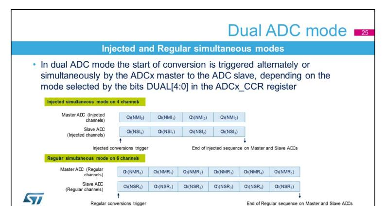
In dual ADC mode, conversions can be started either simultaneously or alternately on ADC master and ADC slave.
