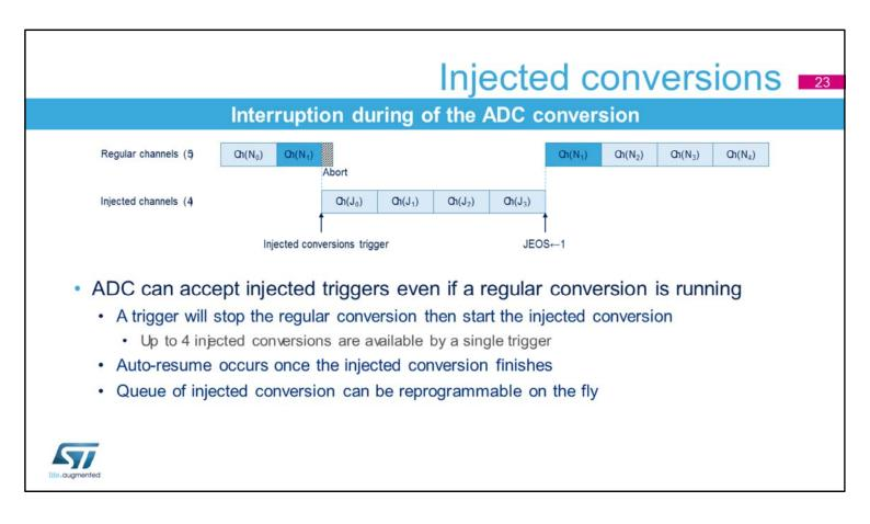
An injected conversion is used to interrupt the regular conversion, then insert up to 4 channel conversions. Once an injected conversion is finished, the regular conversion sequence can be resumed.
