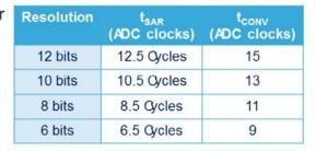
The global conversion time is equal to the sampling time plus the conversion time.
