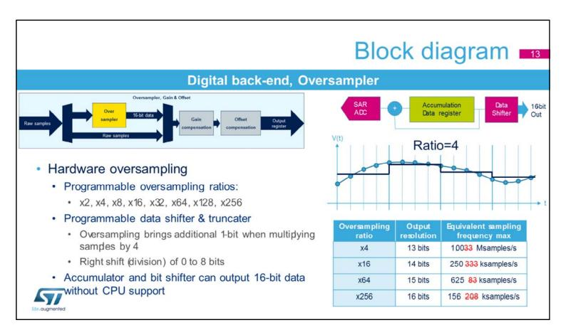
The ADC includes the oversampling hardware which accumulates data and then divides without CPU assistance.
