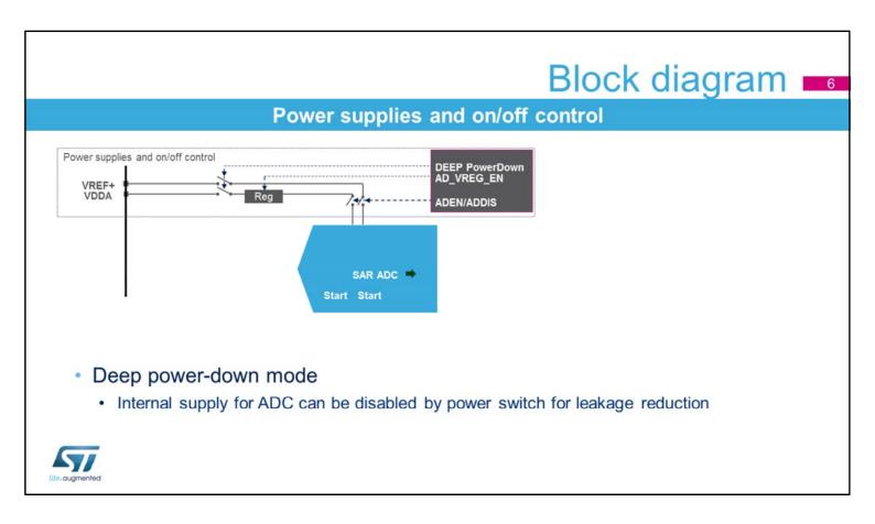
The analog part of the ADC needs two power supplies:
