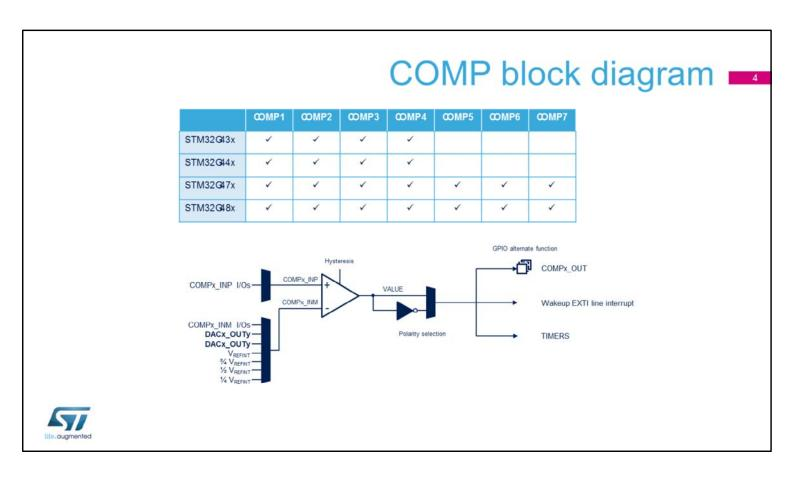
The number of comparators depends on the exact reference of the STM32G4 microcontroller. STM32G43x and STM32G44x series implement 4 comparators while STM32G47x and STM32G48x series implement 7 comparators.
