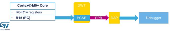
The DWT is used to trigger watchpoint events caused by a match between the current data or instruction address and the contents of comparators programmed by the debugger.
