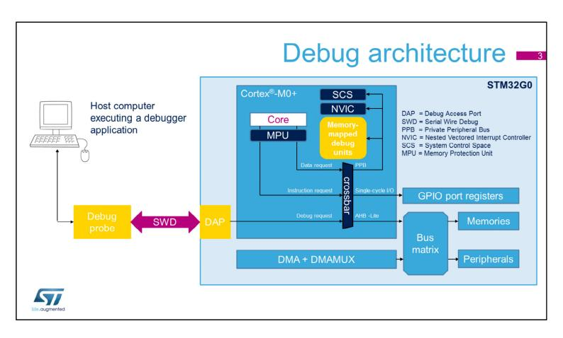
The Debug Access Port (DAP) enables an external debug probe to access any memory-mapped resources also accessible from the Cortex®-M0+ core. Note that the Memory Protection Unit (MPU) does not intercept the requests initiated by the DAP. The Serial Wire Debug (SWD) protocol used to connect the debug probe to the Cortex®-M0+ relies on 2 wires, and is appropriate for the STM32G0, due to its low pincount packages (64, 48, 32 or even 28 pins).
