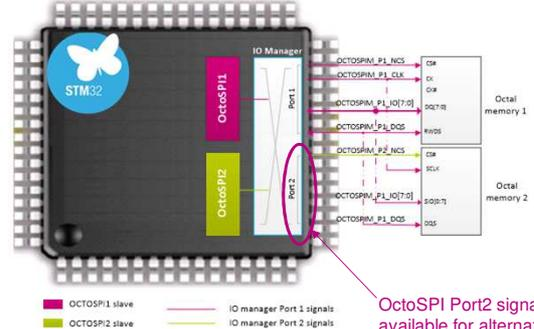
OctoSPI Port2 signals available for alternate signals, except P2\_NCS
