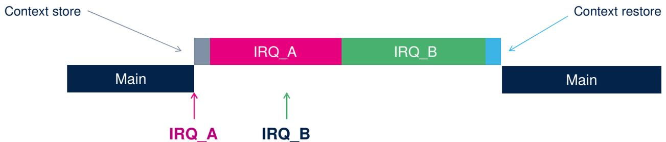
When an interrupt request with lower or equal priority is raised during execution of an interrupt handler, it becomes pending. Once the current interrupt handler is finished, the context saving and restoring process is skipped and control is transferred directly to the new exception handler to decrease interrupt latency.
