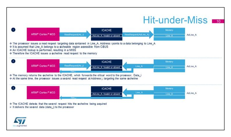
The Hit-under-miss capability is the ability to serve processor requests (access to cached data) during an ongoing line refill due to a previous cache miss.
