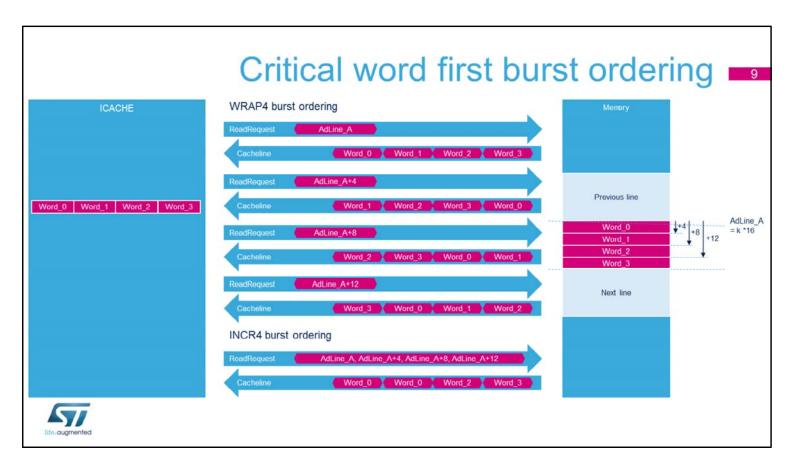
The burst type of AHB memory transactions for remapped regions is programmable: INCR or WRAP.
