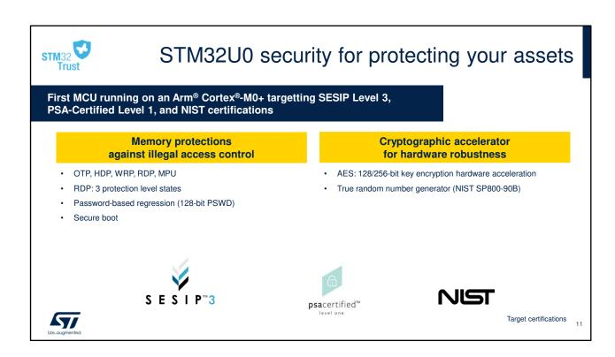
The STM32U0 is based on the Arm Cortex®-M0+ core and targets SESIP Level 3, PSA-Certified Level 1, and NIST certifications.
