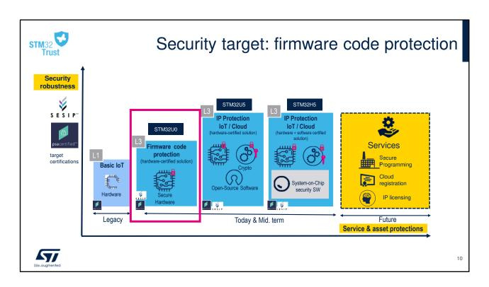
The STM32U0 is the first MCUs with an Arm® Cortex®-M0+ targeting SESIP Level 3 and PSA level 1 focusing on firmware code protection.
