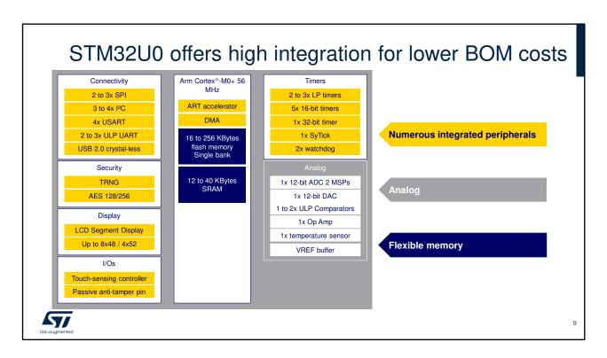
To make this entry-level microcontroller even more compelling, ST maximized the number of integrated peripherals, such as segment display controller, digital-to-analog and analog-to-digital converters, an operational amplifier, and an ultra-low power comparator.
