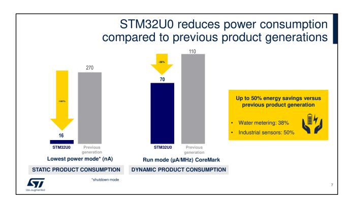
STM32U0 MCUs enable a great leap in energy efficiency through a combination of state-of-the-art design techniques and advanced manufacturing process. These include extremely low static power consumption in standby mode and superior wake-up performance, enabling the MCU to spend more time in power-saving sleep modes to minimize average energy demand. Both static and dynamic consumptions are drastically reduced compared to previous generation's MCUs.
