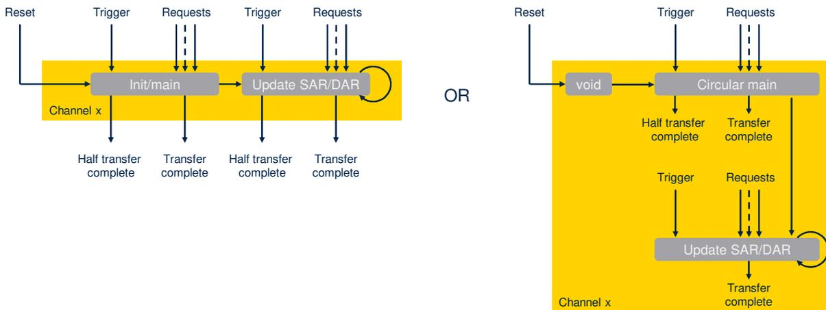
This slide describes the automatic update of the source or destination address register when a unique circular buffer is used.
