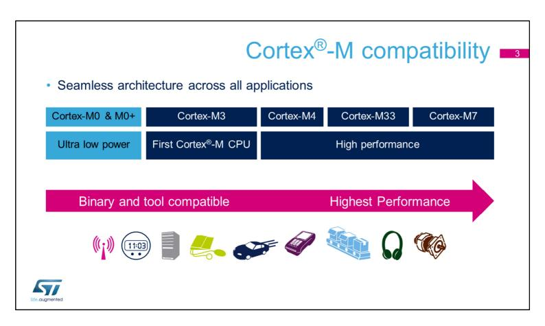
STM32L5 microcontrollers integrate an Arm<sup>®</sup> Cortex<sup>®</sup>-M33 core in order to benefit from the powerful performance of its 32-bit processor architecture and particularly high level of deterministic processing.
