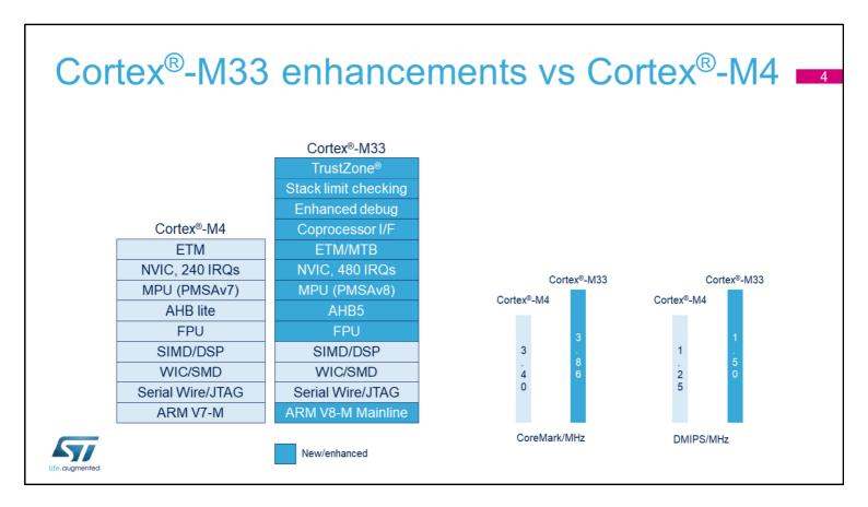
This slide highlights the differences between ARM Cortex-M4 and Cortex-M33.
