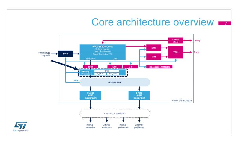
Security attribution and memory protection in the processor is provided by the Security Attribution Unit (SAU) and the optional Memory Protection Units (MPUs).
