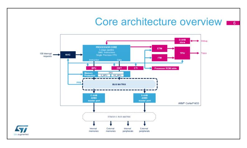
The Cortex®-M33 has neither a cache nor internal RAM. Consequently any instruction fetch transaction and data access is steered to the internal bus matrix. This bus matrix selects the output AHB5 master port according to the address. Two AHB transactions can be in progress at the same time, for instance:
