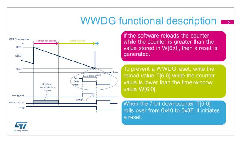
This diagram illustrates how the window watchdog operates. When the 7-bit downcounter rolls over from 0x40 to 0x3F, it initiates a reset. This happens if the application software does not refresh the window watchdog on time. The early interrupt, if enabled can be generated when the downcounter reaches 0x40.
