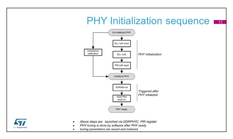
The Complete PHY initialization including SDRAM initialization and DQSTRN is shown in this diagram. The sequence is defined and controlled by the PIR register. This sequence is launched after a system reset. Tuning parameters determined by software during the bring up, are saved and restored.
