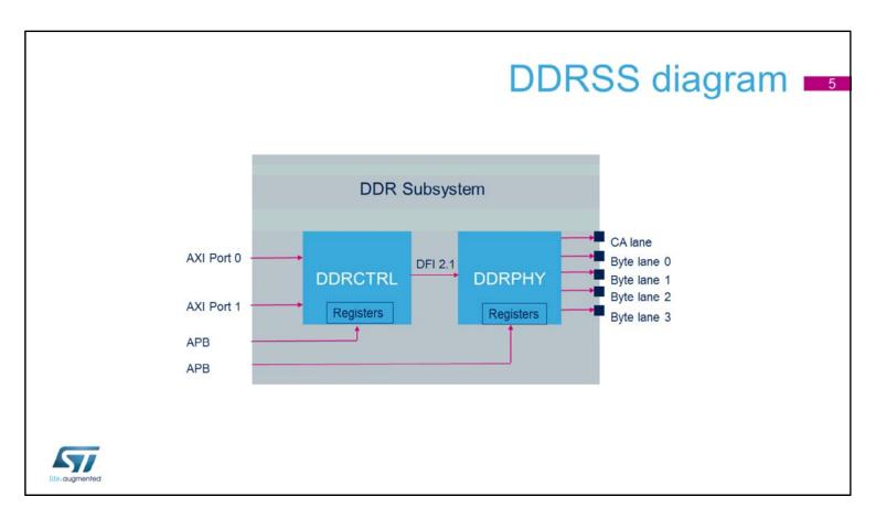
This is a simplified Block diagram of the DDR subsystem (DDRSS)
