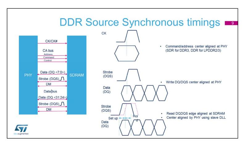
This is a simplified view of a DDR interface using source synchronous signaling. The interface has several signal groups.
