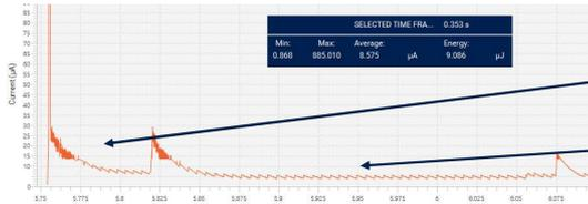
ADC in STOP2 (~10  $\mu\text{A}$ )
