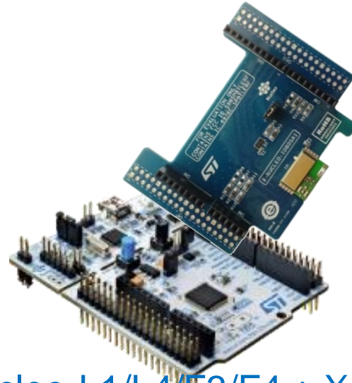
Nucleo-L1/L4/F3/F4 + X-Nucleo-IDB05A1 + X-NUCLEO-IKS01A2 BlueNRG-MS + STM32L1 or STM32L4 or STM32F3 or STM32F4
