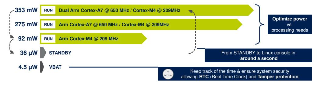
Typ @ VDDCORE = 1.2V, VDD = 3.3V @ 25 °C, Peripherals OFF
