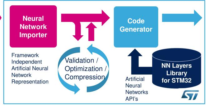
**Embedded Solution Optimized Artificial Neural Network Code** generated for STM32
