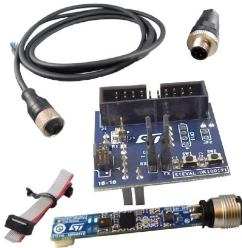
STEVAL-BFA001V1B Stand Alone Sensor Node
