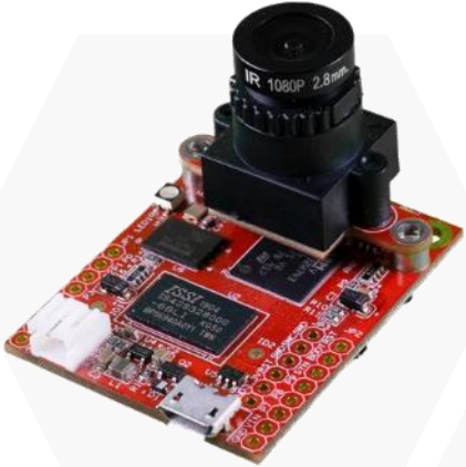
OpenMV CAM Running MicroPython over STM32
