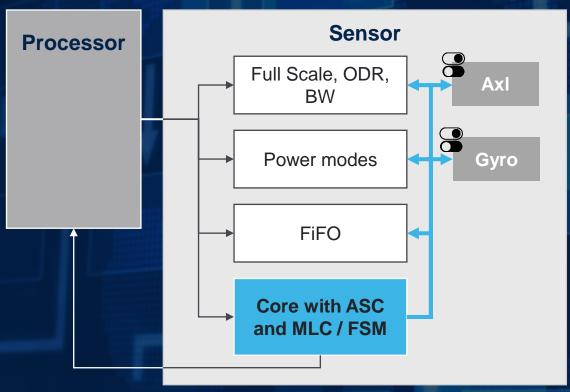
The ASC modifies the sensor settings automatically based on the events detected by the Machine Learning Core or the Finite State machine
