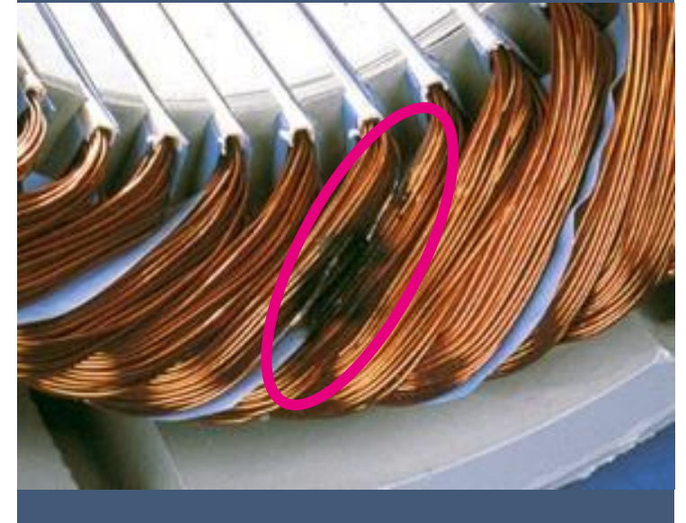
Partial discharge burns the windings
