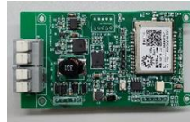
IA.BA 0005.20 KNX-LoRa project based on STM32WL STKNX
