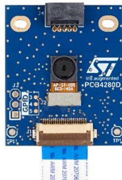
P-Board for integrating turnkey camera modules
