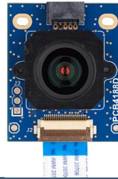
S-Board for integrating sensors with any M12 lens
