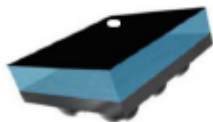
Chip scale package on glass 8 bumps
