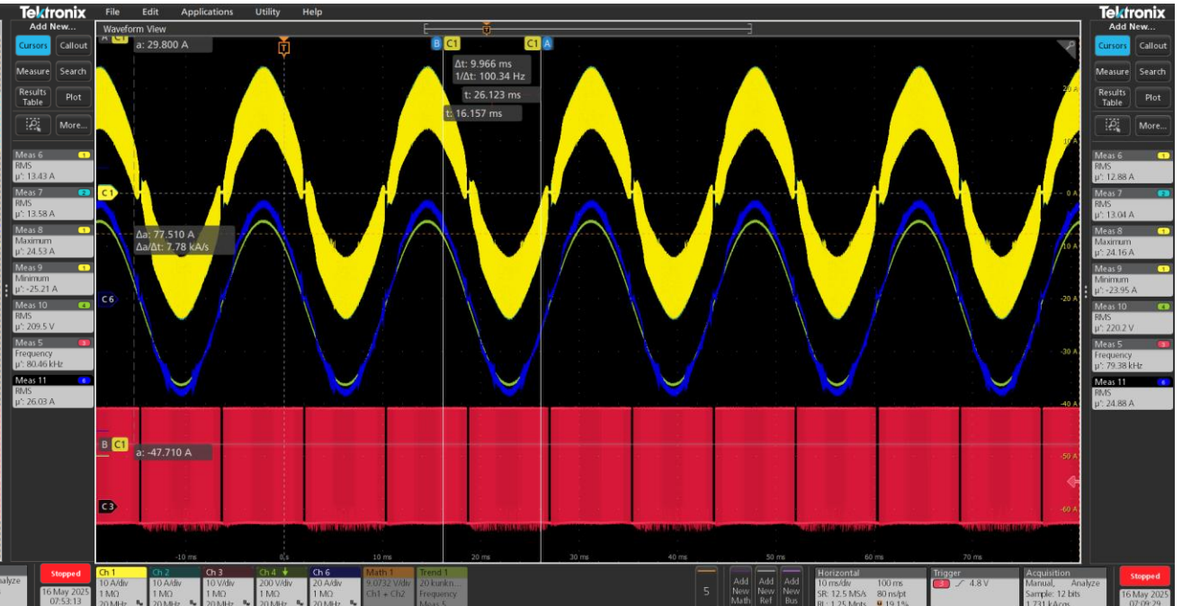
CH1,IL1. CH2, IL2. CH3, HF PWM. CH4, input voltage. CH6, input current at full load 5.5 kW at input voltage 220 V
