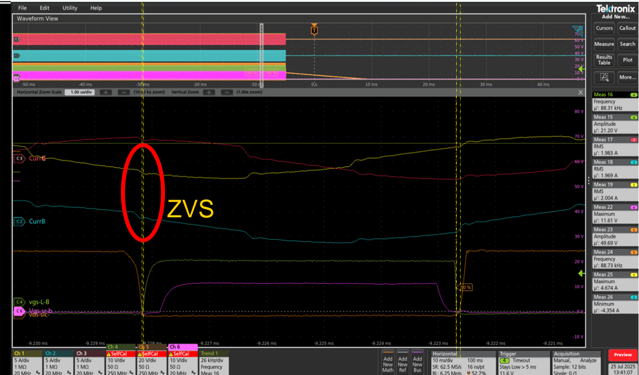
Fig2: Three phase LLC ZVS mode
