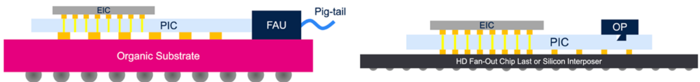
Figure 2: Silicon photonics is the best technology for compact and power efficient optical chiplets on classical organic substrate or more advanced silicon interposer.
