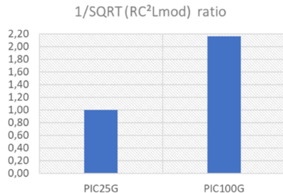
Figure 8: Ratio of our Figure of Merit ( 1/\sqrt{RC^2L_{mod}} ) between PIC25G HSPM and PIC100G HSPM. The modulator length is adapted for an Extinction Ratio of 4.5dB. This figure of merit is directly proportional to the electro-optical bandwidth of the modulator, showing that our PIC100G speed is more than 2 times that of our previous PIC25G industrial platform.
