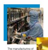
chips is a process of around 400 separate stages in several workshops. Starting with a plain silicon wafer, the Frontend manufacturing results in the etching of several hundreds to thousands of die, depending on the end product and the used technology.
