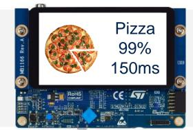
Embedded **image** pre-processing (SW) on the STM32H747
