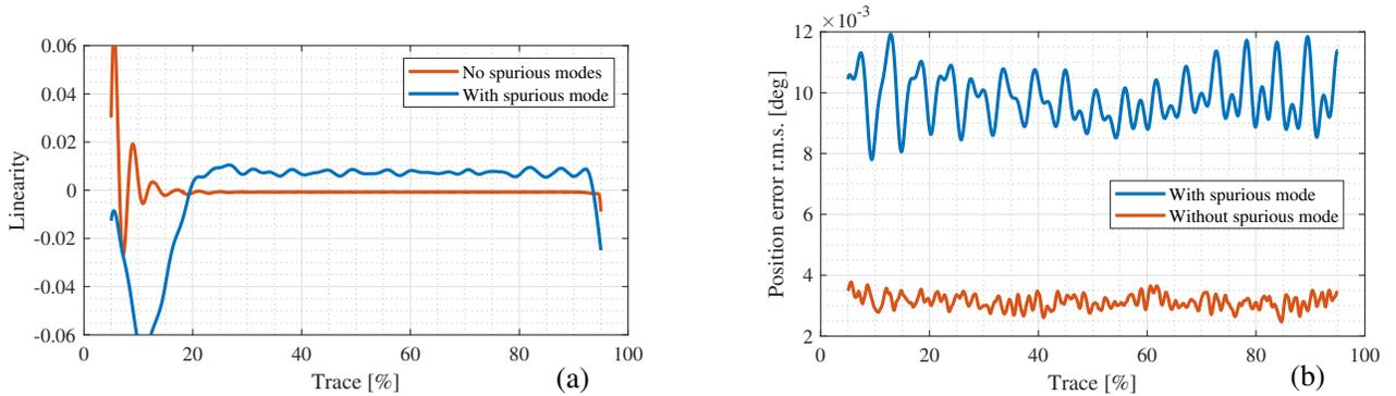
Figure 6. (a) Comparison between the linearity attained with the two simulated mirrors. The RMS of this trace rises from 0.7% when no significant spurious resonance is present, up to 1.82% for the case with a significant mode at 10 kHz; (b) comparison between the reproducibility attained with the two simulated mirrors. The point-to-point RMS position error increases from about  $3 \text{ m}^\circ$  to about  $12 \text{ m}^\circ$  when introducing spurious modes.
