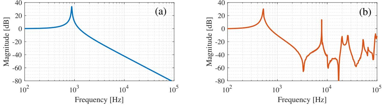
Figure 2. Magnitude of the transfer function from PZT drive voltage to piezoresistive sensor output voltage of an ideal micromirror (a) vs. a real micromirror (b) where significant coupling of high-frequency resonances can be observed. The effect of spurious resonances is modeled as complex-conjugate poles and zeros that can generate even within the control bandwidth.
