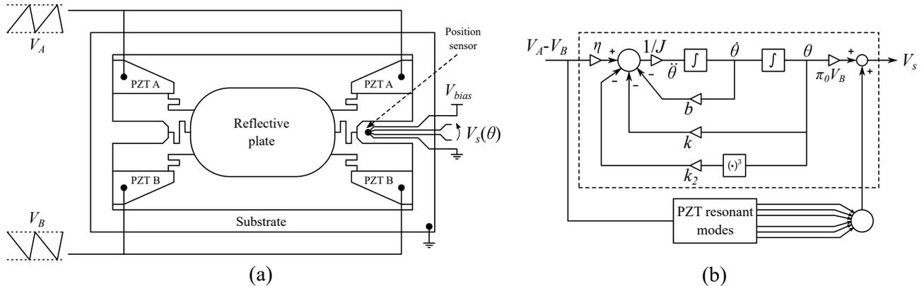
Figure 1. (a) Schematic top-view of a piezoelectric micro-mirror, showing the geometry of the PZT actuators, their electrical connection and the position of the piezoresistive sensor on the MEMS structure; (b) model of a generic piezoelectric micromirror.
