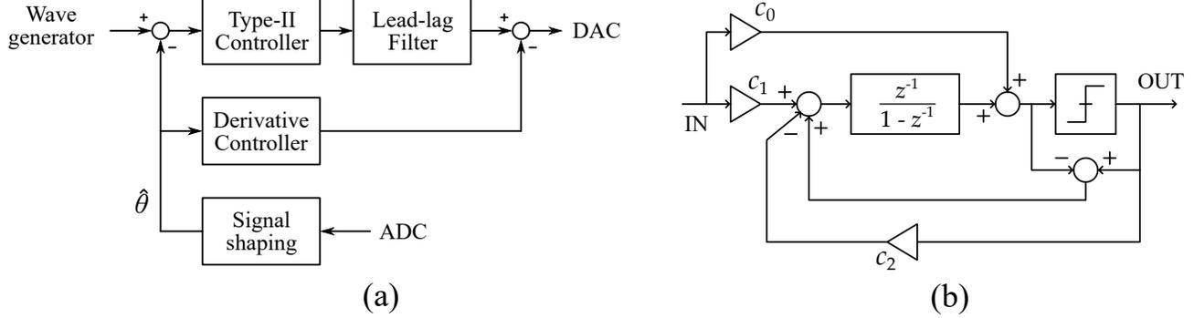
Figure 4. (a) Block diagram of the digital controller, showing the signal shaping block processing the output of the ADC, the “inner” derivative loop, and the position controller constituted by the integrator and lead-lag filter; (b) filter topology used to implement all the controller filters.
