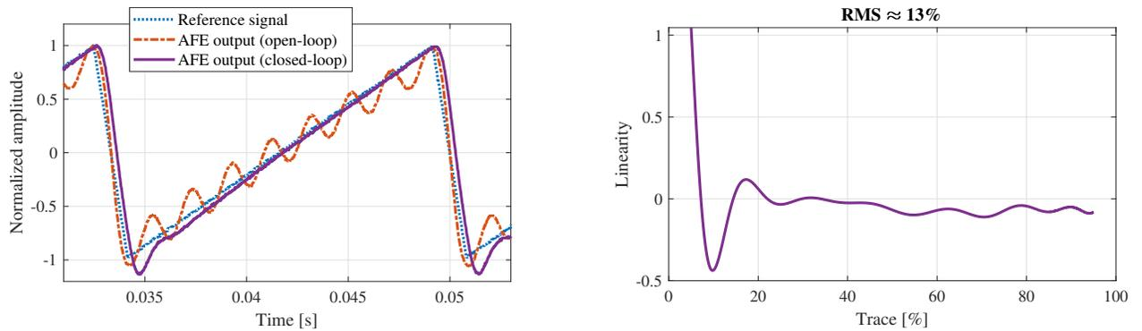
Figure 8. (a) Time-domain normalized response of the analog system. The open-loop and closed-loop waveforms are acquired at the output of the sensor front-end, acquired via oscilloscope; (b) trace linearity extracted from measured data (closed-loop), filtered to remove oscilloscope quantization. Regardless of such quantization, the measured linearity is still quite large, with an RMS in the order of 13%.
