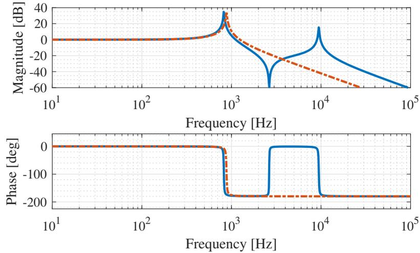
Figure 5. Transfer function of a mirror with no significant spurious modes (dashed orange line), compared to the transfer function of a mirror with a significant mode at about 10 kHz (solid blue line) coupled to the piezoresistive sensor output.
