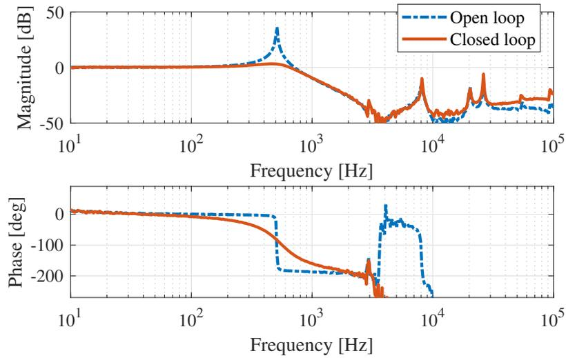
Figure 7. Normalized experimental transfer function (from reference signal to front-end output) in open-loop and closed-loop conditions with an applied derivative controller.
