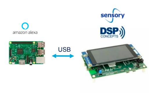
STM32F7 with 2 microphones speech recognition based on Sensory's trigger word recognition and DSP-Concepts audio front end
