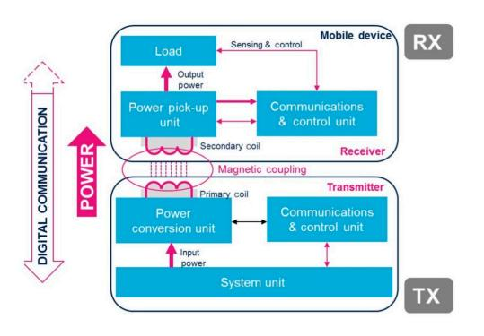
15 Watt solution using STWBC-EP Transmitter and STWLC33 Receiver
