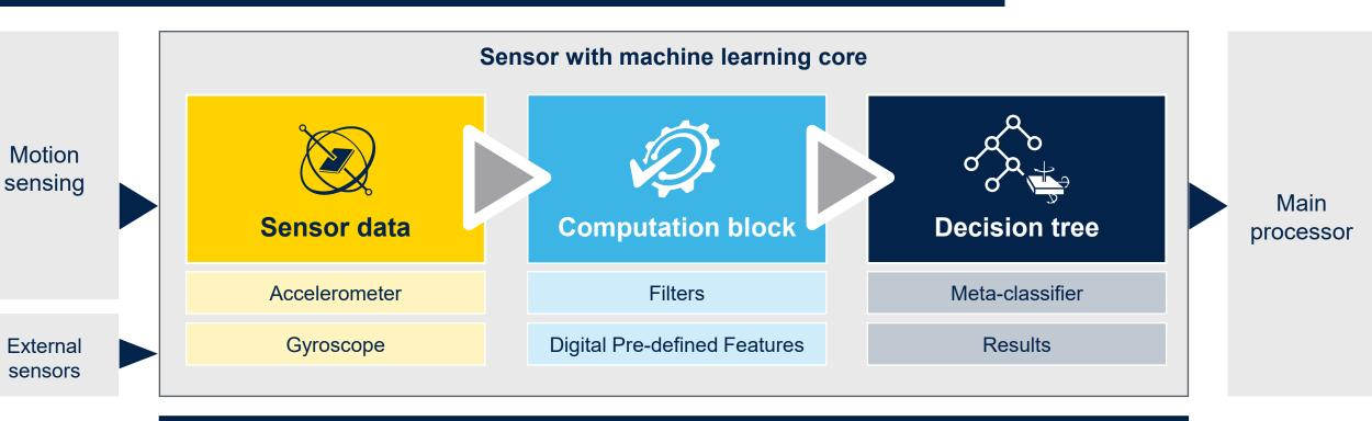
MLC is able to **increase accuracy** with a **better context detectability**, **offloading the main processor** while the built-in sensors identify motion data
