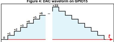
Figure 4: DAC waveform on GPIO15
