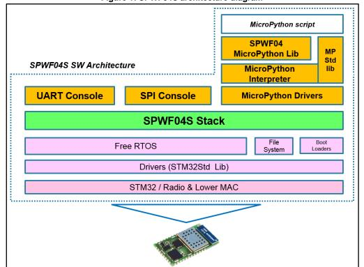
Figure 1: SPWF04S architecture diagram
