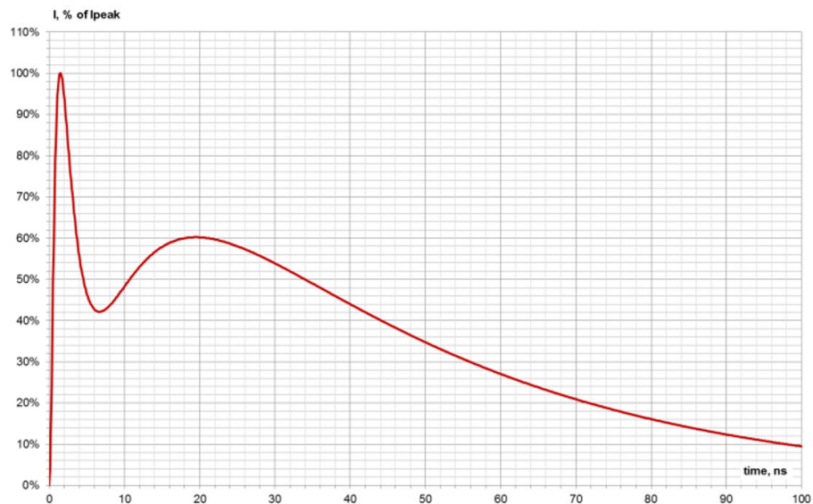
Figure 2. IEC61000-4-2 typical current waveform, contact discharge
