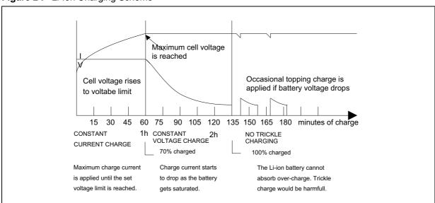
Figure 2: Li-Ion Charging Scheme
