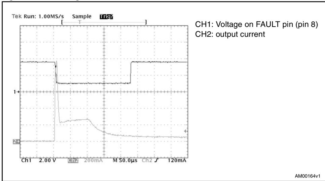
Figure 8. Filter for the FAULT transients
