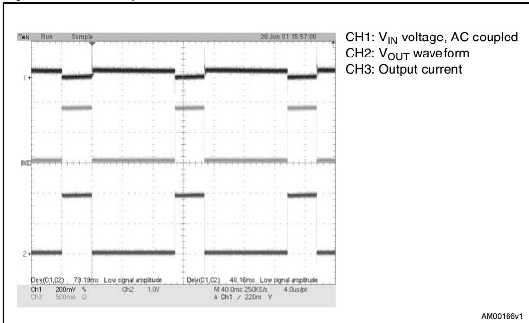
Thermal protection occurs when the junction temperature exceeds 135 °C and the thermal hysteresis is 15 °C. This feature safeguards the device from dangerous currents or temperatures. *Figure 9* shows the thermal protection behavior. The pulse width and period of the output current depend on the thermal dissipation. This test was made in a free air temperature condition.
