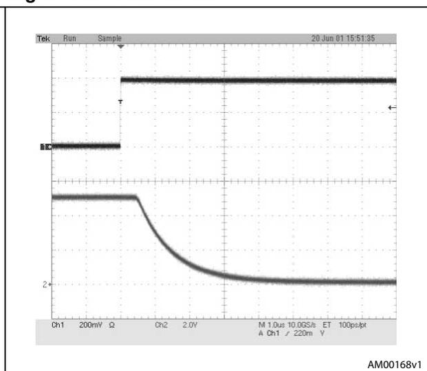
The  $\overline{\text{ON}}$  pin switches over the N-channel MOSFET. [Figure 10](#) and [11](#) respectively show the turn-on and turn-off times.
