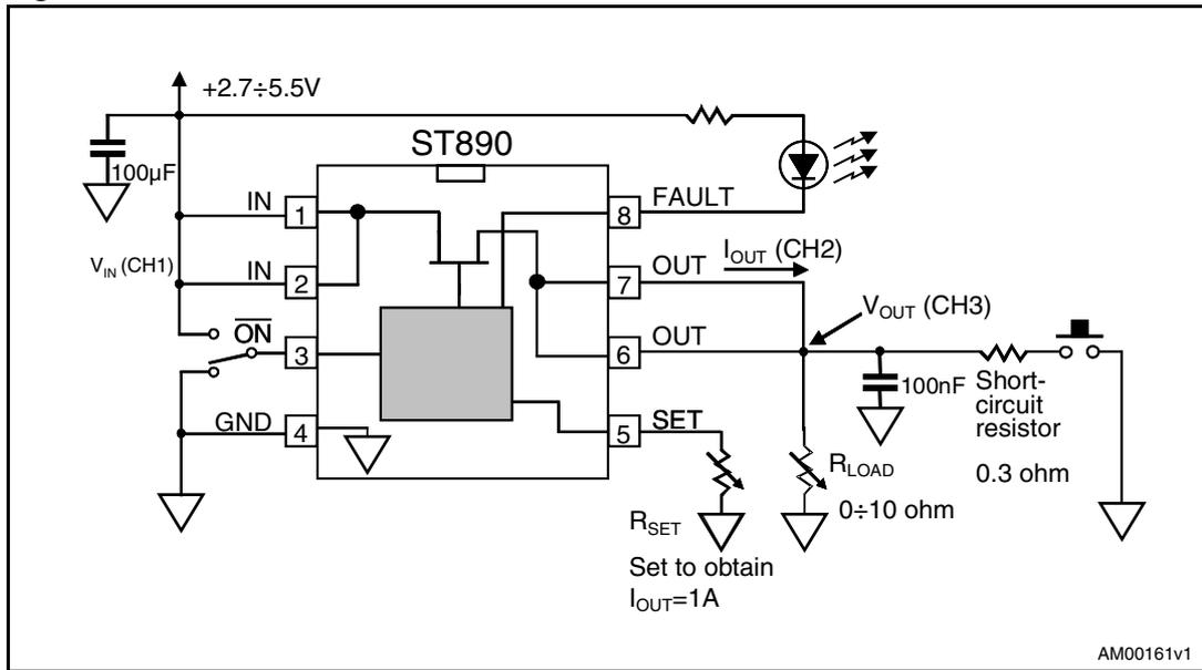
Note: To take this measurement, the input capacitor is 100 µF instead of 1 µF. Typically, a 1 µF input capacitor, like in the demonstration board circuit, is sufficient.
