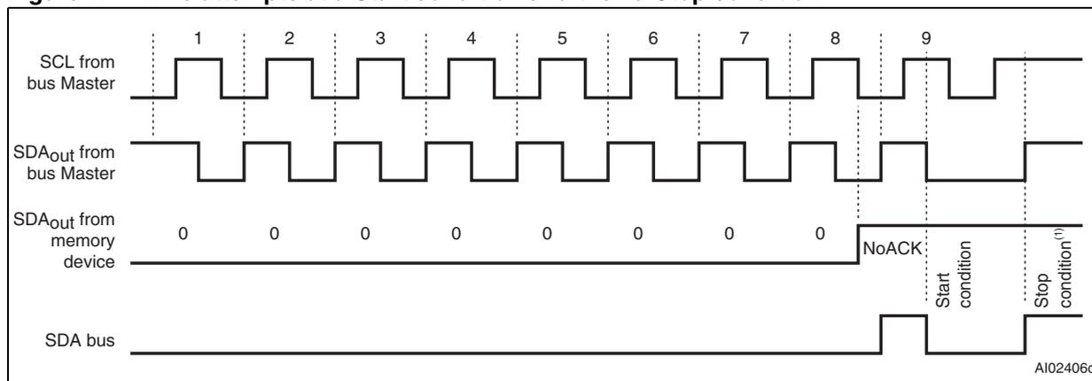
1. The Stop condition following the Start condition sets the M24xxx in Standby mode.
