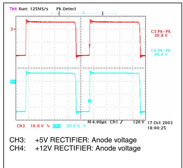
Here following the most salient controller IC signals are shown. In both pictures it is possible to distinguish clean waveforms free of hard spikes or noise that could affect the controller correct operation.
