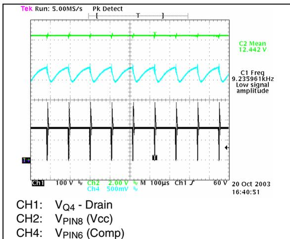
**Figure 10. Standby @230 V<sub>AC</sub> - 50Hz 5V @ 50mA load**
