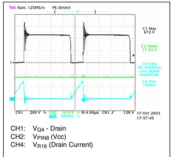
**Figure 5. Maximum rectifiers PIV @Vin = 265 V<sub>AC</sub> - 50 Hz and full load**
