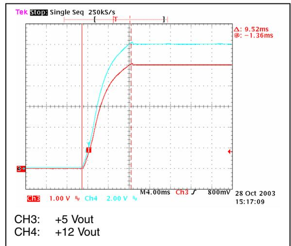
In the above picture the rising slopes at full load of the output voltages at minimum input mains voltage are captured and the rise time is measured. As shown in the pictures, the rising time is monotonic and it is almost constant overall the input mains range. No any overshoot or abnormal behaviour is present overall the input main range.
