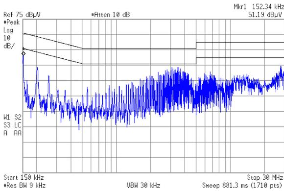
**Figure 25. EN55022 Class-B Peak Measure 230 V<sub>AC</sub> - 50Hz - FULL LOAD**
