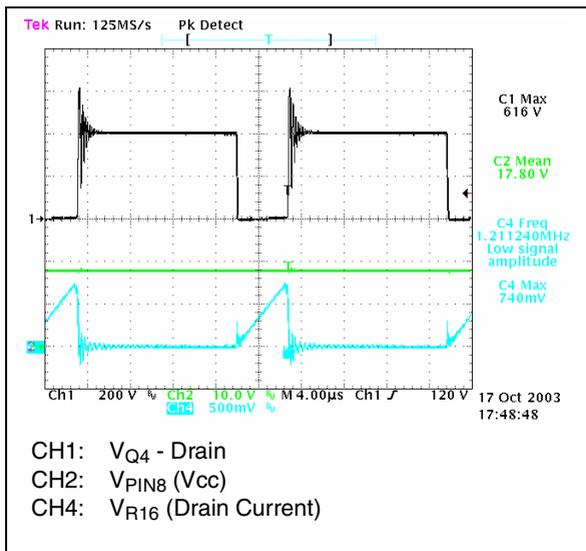
The pictures here above show the drain voltage and current at the nominal input mains voltage during normal operation at full load. As visible, the circuit works in CCM both at nominal high and low mains.
