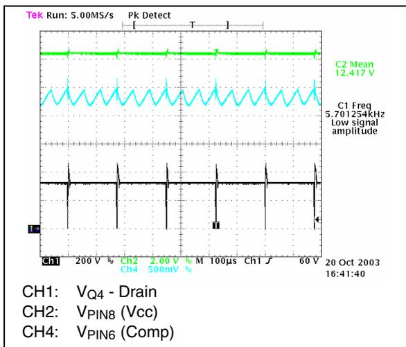
**Output voltage ripple @full load**
