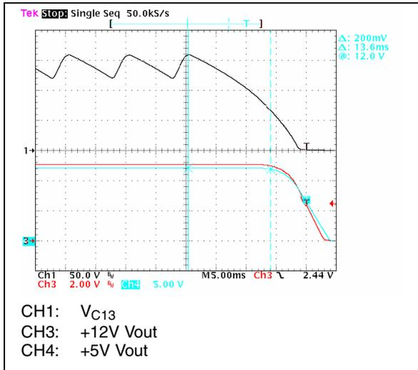
**Short-Circuit Tests at Full Load**
