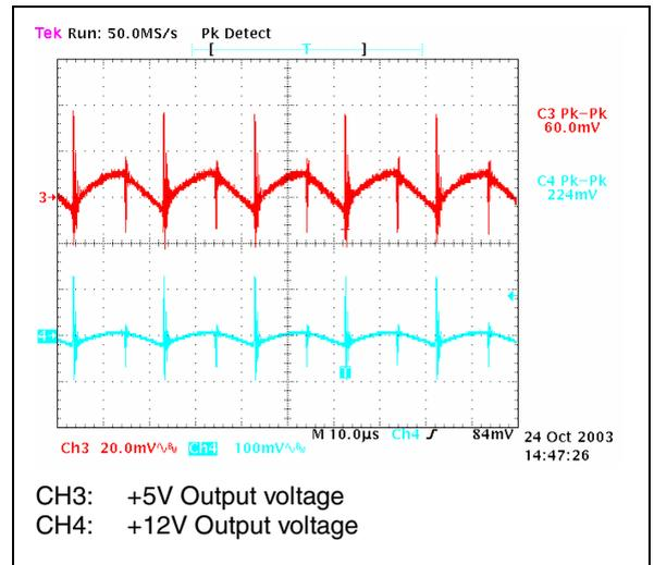
In figure 11 the output voltage ripples at switching frequency are measured. As shown, the ripple and the spikes are very low thanks to the additional LC filters added on both output and avoiding the use of bigger or expensive output capacitors.
