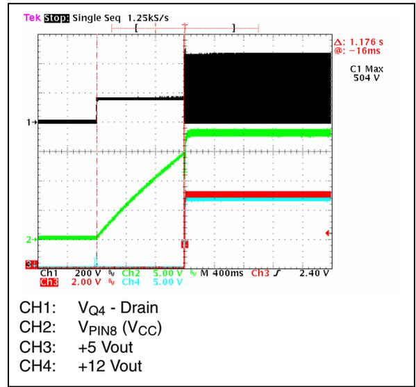
**Figure 15. Start-Up Behaviours @full load -
