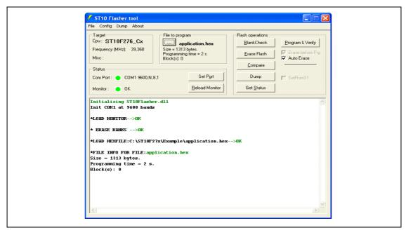
Click on the *Program & Verify* button to trigger the programming operation. Now the loaded hex file is transferred to the ST10 and programmed into the embedded flash memory.
