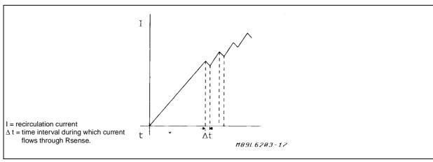
Braking the motor by short-circuiting it involves an accurate study of the mechanical system during the design phase. Knowing the value of the BEMF generated by the motor during braking, the motor resistance, and the equivalent resistance of the MOS and diode involved during recirculation it is possible to determine the recirculation current and if it is less than or greater than the maximum value that the IC can tolerate.
