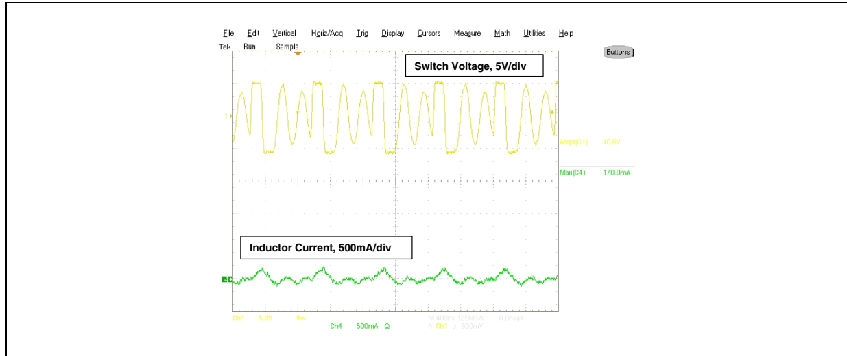
Figure 5. Typical waveform of the switching regulator, 5 V IN , - 5.5 V OUT , no load
