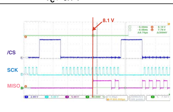
Figure 16. Communication resumes for V_C > 8.1\text{ V}
