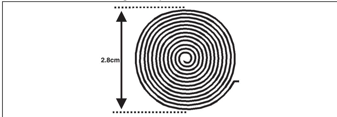
An inductor as described in [Figure 6](#), allows the  $di/dt$  rate to be limited (in case of a spurious firing of the start ACST when the run ACST is already on) below  $60 \text{ A}/\mu\text{s}$  (start capacitor is charged up to  $510 \text{ V}$ ). The semiconductor device operation is then well secured.
