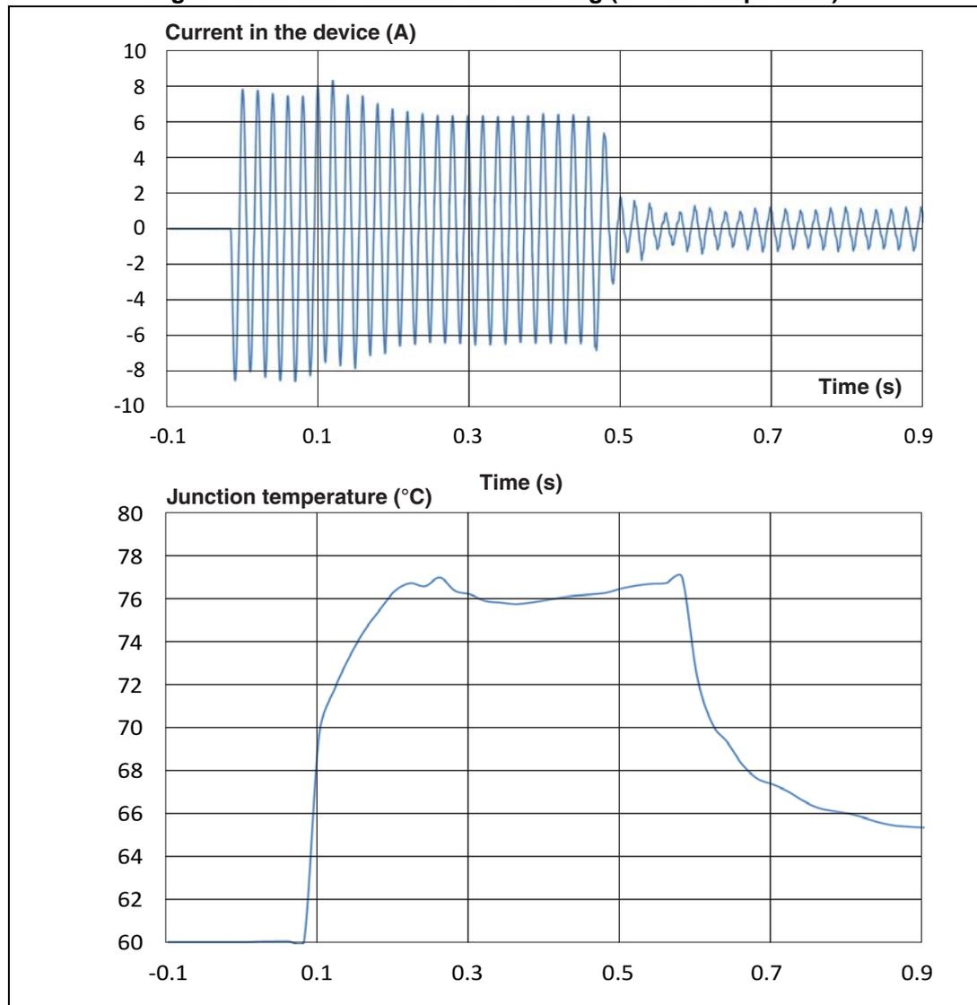
When dealing with the current rating for AC semiconductor switches, the rate of decrease of the current must also be checked. This constraint will depend on the chosen circuit topology.
