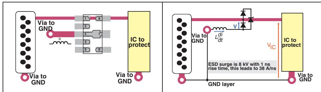
A very simple calculation shows that for a 8 kV ESD surge according to IEC61000-4-2, the overvoltage due to parasitic inductances may be really significant, as shown in *Figure 2*. Assuming that each inductance value is 5 nH (corresponds to metal track 5 mm long):
