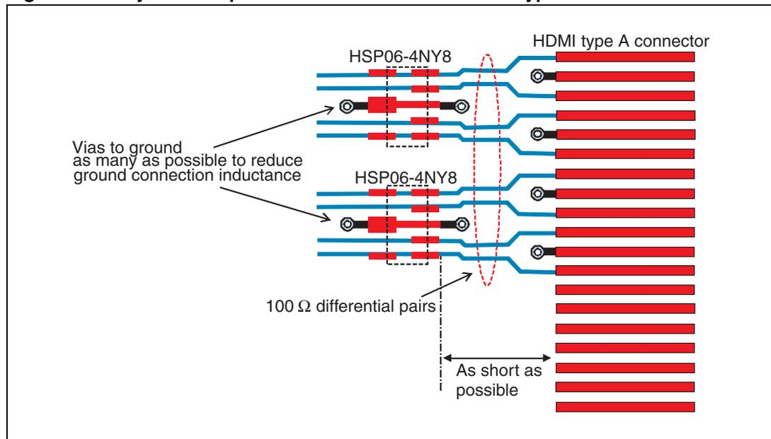
Figure 11 shows an example of PCB layout for HSP061-4NY8 with an HDMI type C SMD connector
