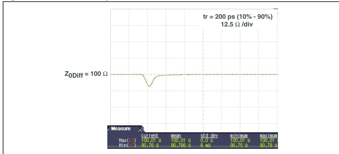
Figure 7 shows the differential impedance measured with the “Time Domain Reflectometry” method. This method consists of sending a pulse with a short rise time (200 ps between 10% and 90% for HDMI) and to measure the reflected pulse. This gives the impedance of the line along the signal path.
