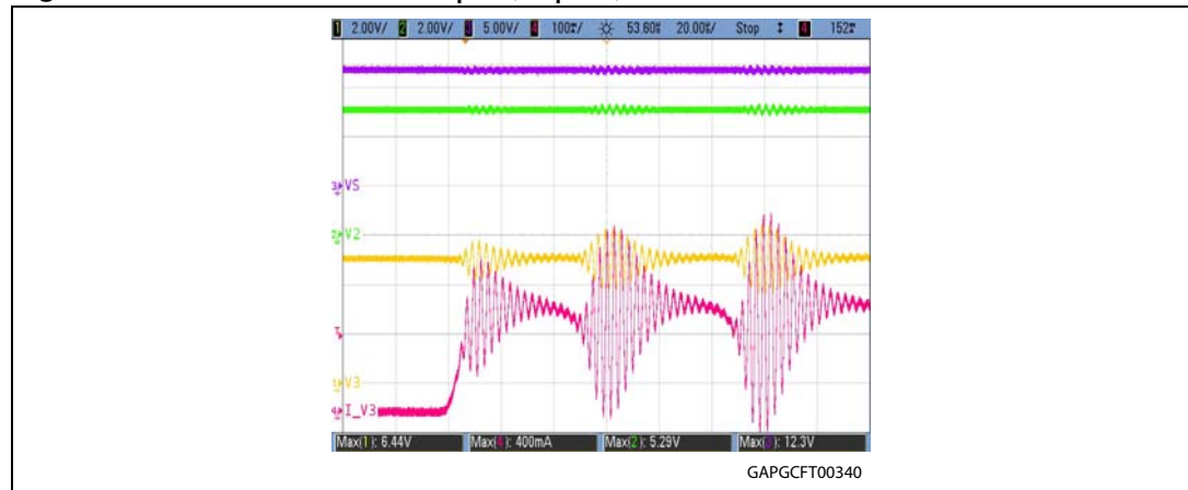
Figure 14. Combination n°1 - C i = 0; C 1 = 0; load switch ON
