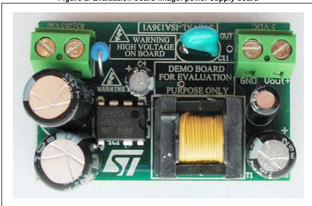
Figure 1. Evaluation board image: power supply board
