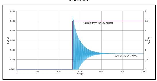
Figure 5: OA1MPA output response to a small current signal without feedback capacitance, Rf =  $8.2\,\mathrm{M}\Omega$
