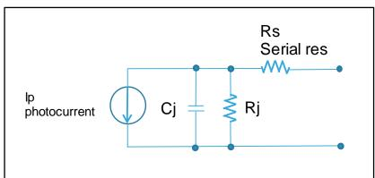
Figure 3: Equivalent circuit of UV sensor
